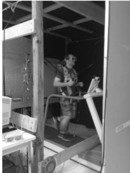
Figure 1: Setup for the Virtual Reality Locomotion Interface, Including Treadmill and Projection
